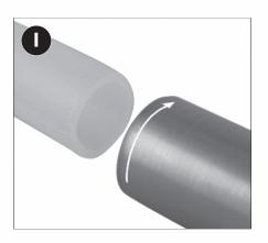
I Attach the foot valve to the plastic tubing by threading the foot valve clockwise (right hand thread) on the tubing as far as possible. The threads on the foot valve will self-tap into the tubing to provide a strong, water tight connection. Test the connection by pulling vigorously on the foot valve.
