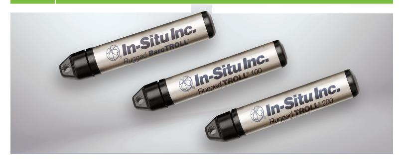
RUGGED TROLL 100 AND 200 DATA LOGGERS ARE DESIGNED FOR LONG- AND SHORT-TERM GROUNDWATER AND SURFACE WATER MONITORING. THESE NON-VENTED (ABSOLUTE) WATER LEVEL DATA LOGGERS MEASURE AND RECORD CHANGES IN WATER LEVEL, PRESSURE, AND TEMPERATURE. ENSURE ACCURATE RESULTS BY USING A RUGGED BAROTROLL® DATA LOGGER. ALL LOGGERS ARE COMPATIBLE WITH THE USER-FRIENDLY VUSITU™ MOBILE APP AND WIN-SITU® PC SOFTWARE.
