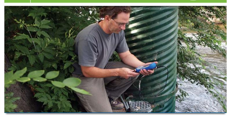
Collect, store, analyze, and transfer data using the versatile RuggedReader Handheld PC. When connected to In-Situ® Inc.'s water level or water quality instruments, the RuggedReader Handheld PC functions as a reliable, easy-to-use data management system. Durable construction stands up to regular field use and harsh conditions.
