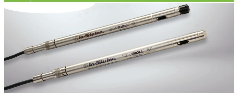
MEASURE AND RECORD WATER LEVEL, WATER PRESSURE, CONDUCTIVITY, AND TEMPERATURE WITH THE AQUA TROLL 200, OR ONLY CONDUCTIVITY AND TEMPERATURE WITH THE AQUA TROLL 100. UNIQUE CONDUCTIVITY CELL ALLOWS FOR A WIDE, ACCURATE MEASUREMENT RANGE IN A NARROW DIAMETER INSTRUMENT (SUB-1 INCH).
