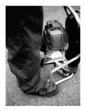
4. During pumping it is recommended that the operator pins the frame legs to the ground with one or both feet.
