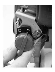
The Stop/Start switch is located on the side of the engine, near the fuel tank filler cap. (See picture)
