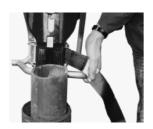
1. Lift PowerPack and hook onto the lip of the borehole lining or headworks (see picture).
