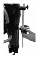
7. Withdraw inertial pump tubing to the required height above the base of the borehole. Pass the tube fully through the appropriate aperture in the tubing clamp (options are for Standard or High Flow tubing) and pass it through the tube guide at the top of the pump body (see picture). We recommend tubing is clamped to the left-hand side of the clamp.
