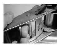
Squeeze the ratchet release slide and rotate the handle anticlockwise until it engages in the slots provided (see picture).
