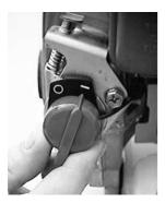
Start/Stop Switch: In an emergency, to switch off engine, turn knob to off position (O).
