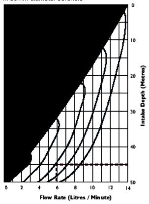
**High Flow System** in 100mm diameter borehole
