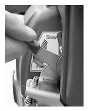
1. Position the throttle control lever fully to SLOW. This stops the actuator operating.
