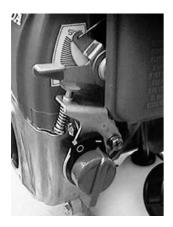
The throttle control and the Stop/Start switch are located on the side of the engine, near the fuel tank filler cap. (See picture)
