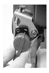
2. Turn the engine switch to the off position (0).
