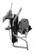
6. Ensure the tube clamp is positioned over the centre of the borehole by rotating the locking disc on the clamp arm in or out to align with the centre of the borehole lining (see picture).
