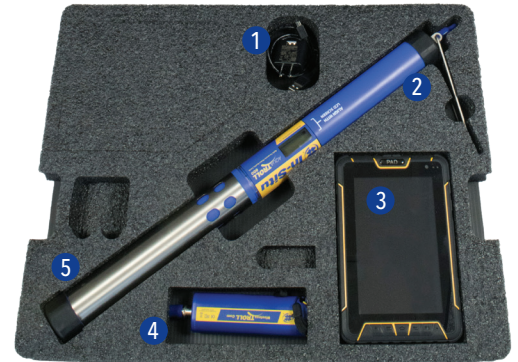
1) Micro USB charger for Android tablet and Wireless TROLL Com; 2) Aqua TROLL 600 Multiparameter Water Quality Sonde (batteries included); 3) Android tablet w/ VuSitu App; 4) Wireless TROLL Com with carrying case and belt clip; 5) Integrated calibration clip
